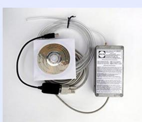
Figure 1: The INFILTEX INFRA 20 amateur infrasound detector
