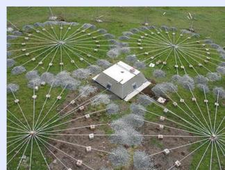
Figure 2: One node of an international monitoring system infrasound detector. The microbarometer is housed in the semi submerged box, which is connected to a large network of porous hoses
